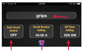
From here tap the gear icon on the right and this will take you to the configuration page. To name the circuit, just tap the default circuit name and a
