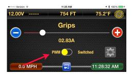
the right. There's also a switch just below the amperage indicator that allows you to set the circuit to be variable or switched.
