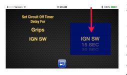
set this tap the "Off Timer Setting" box and another scroll wheel will appear. Here you have a choice of "ignition", which means the circuit will shut down when the ignition is shut off, or you
