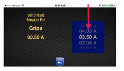
simply tap the circuit breaker setting box and a scroll wheel will appear. Twirl the scroll wheel to 3.5 amps and press the return arrow.
