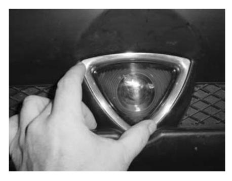
7. Once the lamp assembly is secure in the recess, it's time to run and attach the wiring. Open the trunk. You'll need to remove the black back inside trunk panel and the jack/tow hook locker at the back bottom of the trunk.
