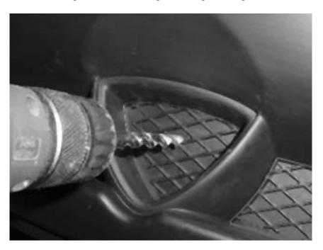
3. Use a small drum sander on a tool like a Dremel to enlarge the opening for the housing. A Dremel makes quick work of this, but a round file with an aggressive pattern will work as well. A template of this hole is provided, but you may need to adjust slightly for your particular assembly.
