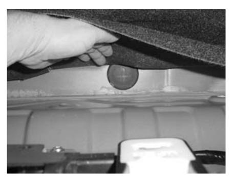
13. Poke two small holes in the rubber plug and insert the two wires from the lamp assembly through the bottom of the plug and out the top.
