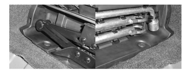
10. Underneath the jack is a 10mm bolt that needs to be removed. In the picture above you can see clips similar to those used to retain the rear trunk panel. These clips (one per side in the jack locker) also need to be removed. Once the bolt and clips are removed the jack locker can be removed.
