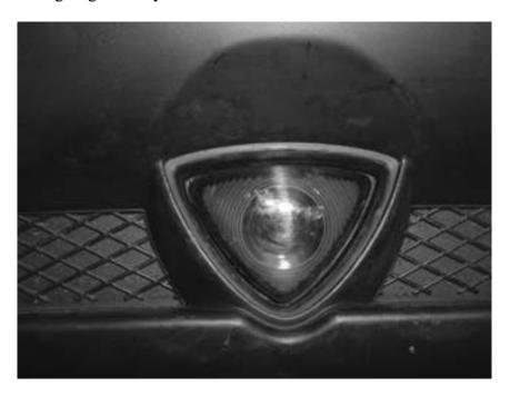
6. Next, if you are installing the unit on a car with the OEM rear accent, carefully install that rear accent around the rotary lamp housing per the OEM instructions. Be careful not to scratch the lens assembly. Use firm but gentle pressure to mount the rear accent. If not, go to step 7.
