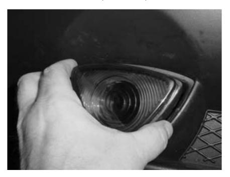
5. The lamp housing should slip easily into the recess once the hole is large enough. Do not force the lamp housing into the recess, as you may damage the housing. It is a very simple form fit and requires no pressure to seat the housing.
