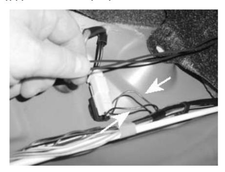
16. Using the two wire tap clips provided, tap into the two wires identified above. You'll probably want to trim any excess wire before making the tap. CAUTION: double-check to make sure there is enough wire under the bumper to allow the lamp assembly to plug into the lamp housing BEFORE making any final cuts.
