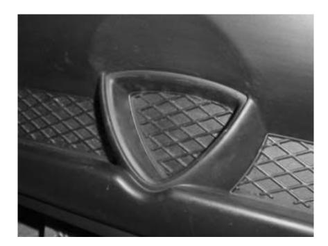
2. Drill a large (3/8") hole in the center of the recess so that the drum sander or file can be used to enlarge the hole to accept the lamp housing.
