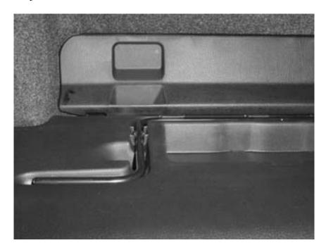
8. There are 4 retaining pins (2 per side) that hold the rear trunk panel in place. Remove those pins by popping the center of the pin out to release it, then you can remove the entire pin. Once the pins are out, the panel lifts up and out.
