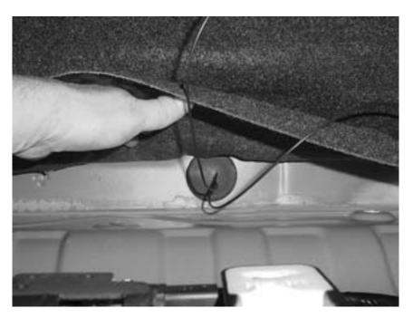
15. Locate the connector where the wire leading to the license plate lamp is plugged in. There are two wires coming out of the top of that connector that will be used to supply power to the rear rotary lamp.
