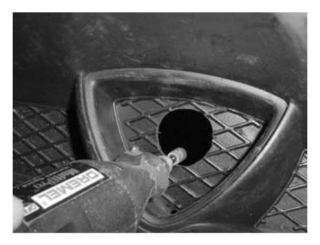
4. Check for fit of the lamp housing in the recess and hole you have cut. If more material needs to be removed, take your time ... you're almost there.
