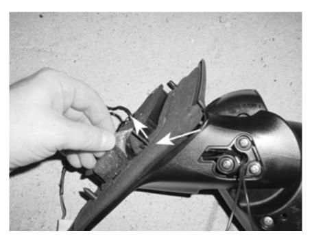
33. Once the wires have been run as indicated, the panel under the mirror assembly can be replaced
