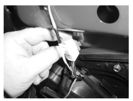
23. To remove the mirror assembly from the car you need to remove the three (3) 8mm screws located behind the speaker panel in Step 6. As you loosen the third screw, be sure to hold the mirror assembly so it does not accidentally fall to the floor. Carefully remove the mirror assembly from the door. CAUTION: There are plastic pins in the mirror housing used to locate the mirror assembly on the door. These pins can break if you are not careful removing the mirror assembly.
