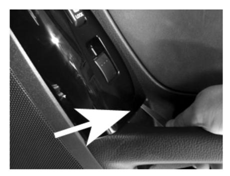
13. Once the panel is free at the bottom, carefully pull it out. NOTE: There is a small plastic clip at the top of this panel. Be sure to carefully pull the panel away to avoid snapping the clip.
