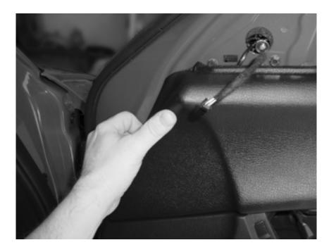
17. Once the nine clips are released, the door panel can be pulled off the door by lifting it straight up. The door panel "hangs" on the window opening so it needs to be lifted off the window opening to come free. CAUTION: There are still two wire assemblies that need to be disconnected before the door panel will be completely free. You just want to lift the door panel off the door.
