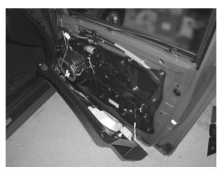
19. There is a small LED light that illuminates the door switches at night. You need to disconnect this wire assembly at the connector indicated by the arrow.
