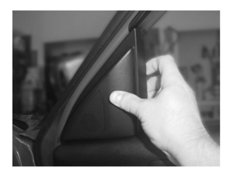
8. There is a wire and connector (see arrow) running to the speaker. You'll need to disconnect the connector (there is a small tab) to release the speaker housing and assembly
