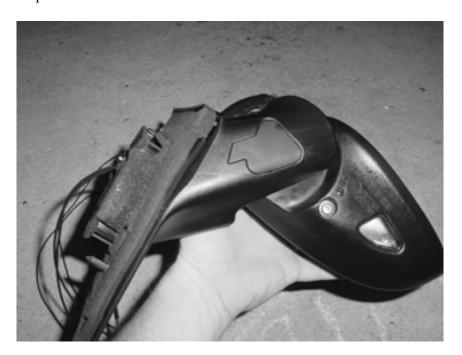
34. There is a retaining screw in the center of the mount panel. Loosen this screw and run the wires under the flat washer and re-tighten the screw. CAUTION: DO NOT OVERTIGHTEN THE SCREW AND CRUSH THE WIRES. Just make it snug to hold the wires in place.
