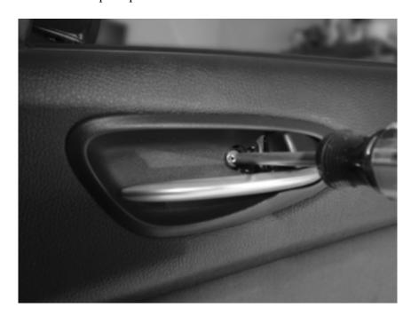
11. You can then remove the cover. You may need to pull on the handle just a bit to aid in removing this small cover.
