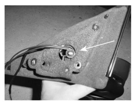
35. Replace the mirror on the doorframe using the three 8mm bolts previously removed. Plug the mirror wiring harness back into the socket from step 22. Run the puddle lamp wire assembly through the access hole and along the path shown to the courtesy lamp at the back of the door.
