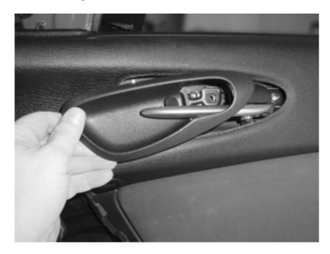
12. Next, you need to pry out the bottom of the window switch/door lock panel. Use a screwdriver covered with a small amount of masking tape to avoid scratching the piano black finish. Carefully pry the base away from the armrest/handle panel.
