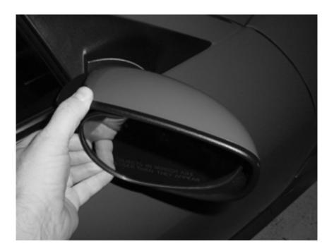
4. Three ball/socket connectors packed in grease hold on the mirror. You must continue pulling on the mirror to extract it from all three sockets
