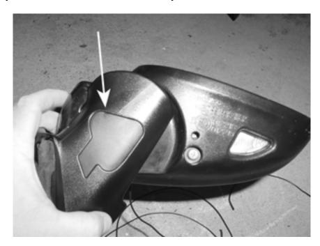
30. Run the two wires from the puddle lamp down the cable run and out the other side.
