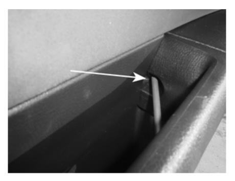
16. With all three screws now removed, you are ready to pull the inner door panel loose. There are nine (9) clips that hold the door panel. Working your way around the perimeter of the door, pull the panel to pop out the clips. CAUTION: DO NOT TRY TO COMPLETELY REMOVE THE PANEL AT THIS TIME. YOU ONLY WANT TO RELEASE THE NINE CLIPS.
